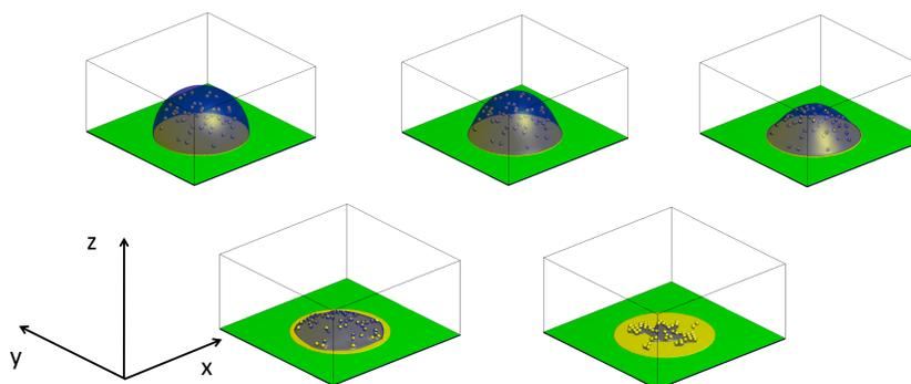
For rough surfaces, experiments reveal that the contact line can remain pinned during drop evaporation until the receding contact angle is reached. The LBM simulation above demonstrates this effect for a receding contact angle of 15°. Like experiments, suspended particles inside the liquid are observed to flow towards the contact line in the LBM.
