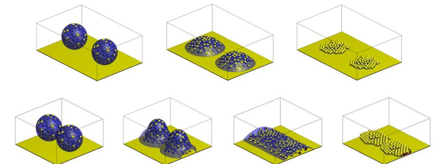
A large spacing between successive drops (top row) leads to isolated deposits. When the spacing between the drops is reduced (bottom row), the spreading contact lines of adjacent drops connect with each other and the final deposit shows continuity. Reducing spacing between drops can lead to line deposits.
